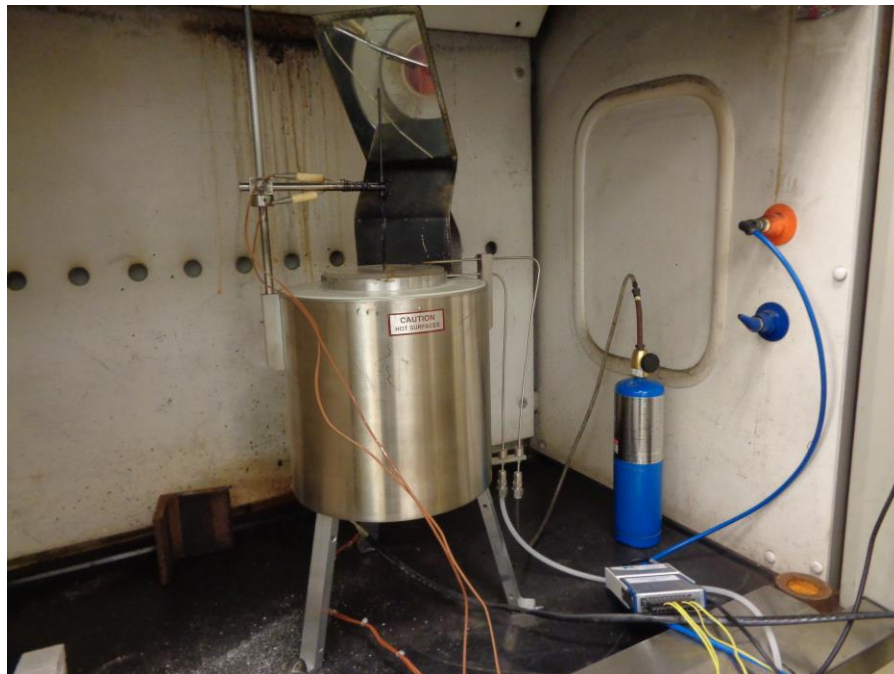
Photo No. 2 Test Furnace Set-up
